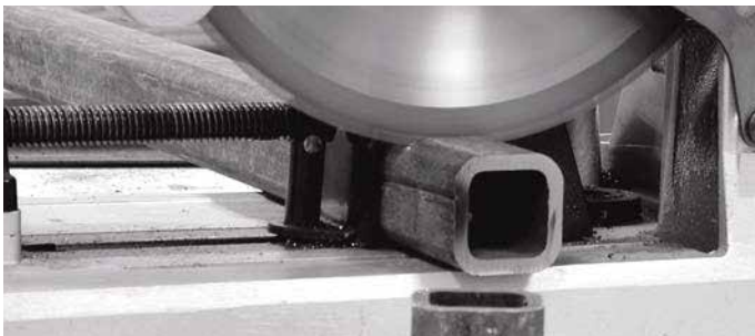
Carbide-Tipped Blades make Virtually Spark-Free Cuts
